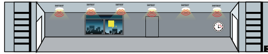
3. No motion is detected in detection area, all lamps synchronously dim to a low light level after hold time.
